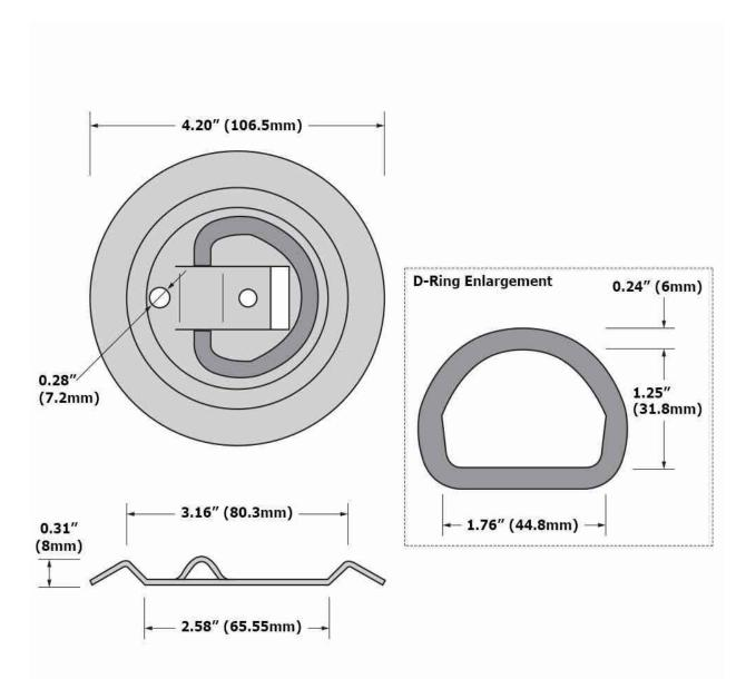
Assembly Break Strength:800 lbs. Working Load Limit:266 lbs. Product Weight:0.3 lbs. Material:316 Stainless Steel
